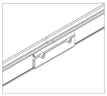
**4.** Connect multiple rails by using rail splice (if required per system design)
